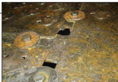
FIGURE 15. Improper assembly of column internals can lower fractionation efficiency
