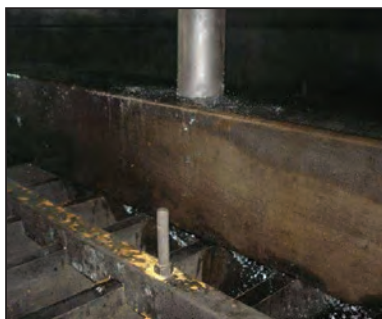
FIGURE 19. When flow is increased above design values, poor distribution of liquid results in the gravity flow distributor
