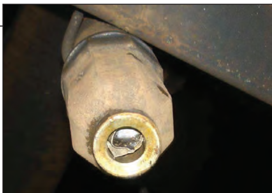
FIGURE 1. Check nozzles for plugs. This one is blocked with a piece of packing
